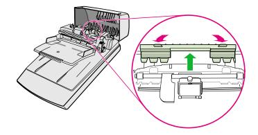
**Note:** Using force to remove the page might cause damage to your originals. If the majority of the paper is already through the main roller, use the procedure to clear jams at the end of a page.
